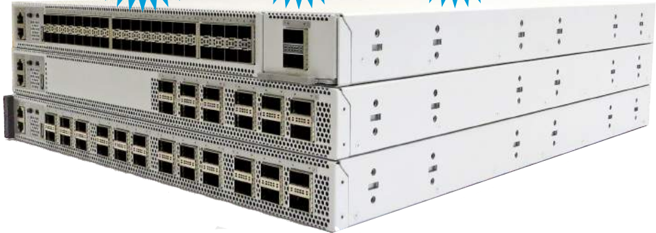
Front to back airflow with N+1 Modular Fans
